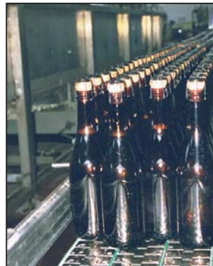
uni SS 881 TAB-K325 Side flexing Beer bottles 3 track Lubricant: Soapy water
