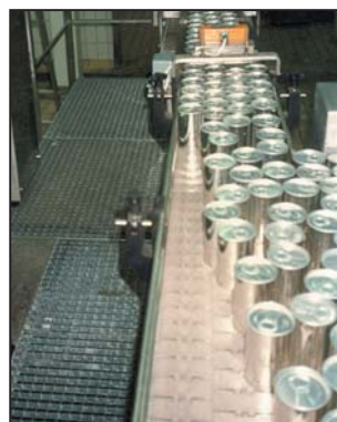
uni 820 K325 Straight running Can accumulation
