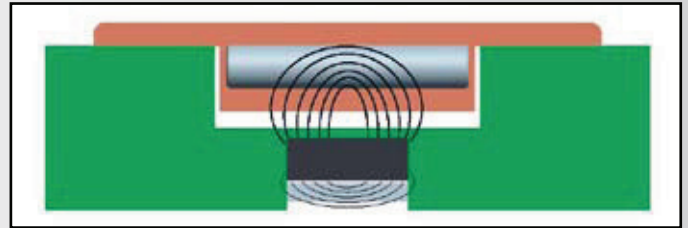
USUAL MAGNETIC CURVE WITH ONLY 1 MAGNET
