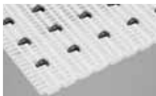
SERIES 900 INSERT ROLLERS • Center-driven • Open hinge • 1.07 in. (27.2 mm) pitch
