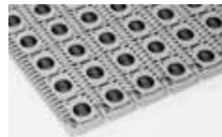
SERIES 400 0° ANGLED ROLLER • Center-driven • Closed hinge • 2.00 in. (50.8 mm) pitch
