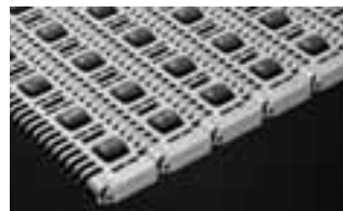
SERIES 400 0.85" TRANSVERSE ROLLER TOP • Center-driven • Closed hinge • 2.00 in. (50.8 mm) pitch
