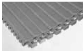
SERIES 2400 • Hinge-driven • Open hinge • Sideflexing • 1.00 in. (25.4 mm) pitch
