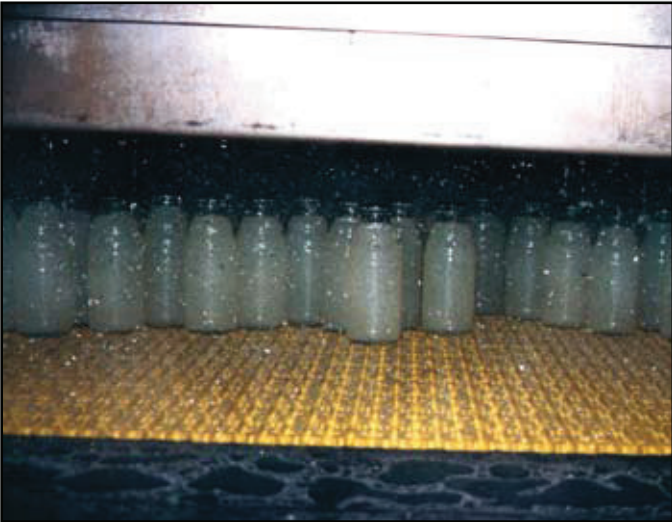
BOTTLE PASTEURIZER INFEED WITH 2500 BELT
