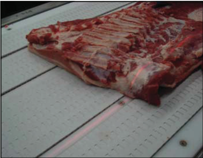
515 BELT ON INFEED OF AUTOMATIC PORK TRIMMER
