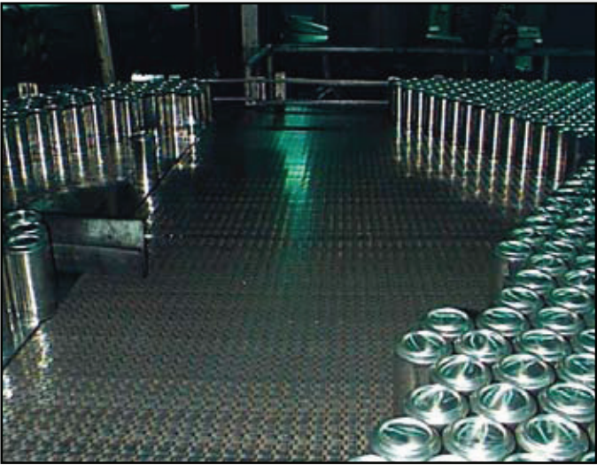
CAN WASHER DISCHARGE WITH 5936 BELT
