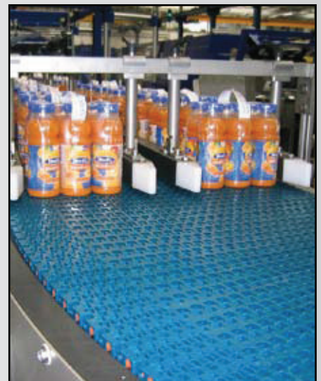
BOXES CONVEYED THROUGH CURVE WITH 1285 BELT
