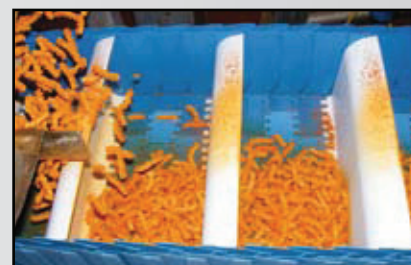
INFEED OF INCLINED CONVEYOR WITH 2010 ISR6
