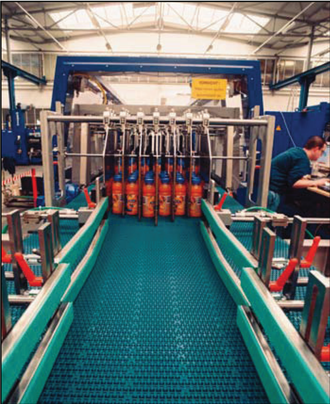
SMALL BOTTLE CONVEYOR WITH 500 BELT
