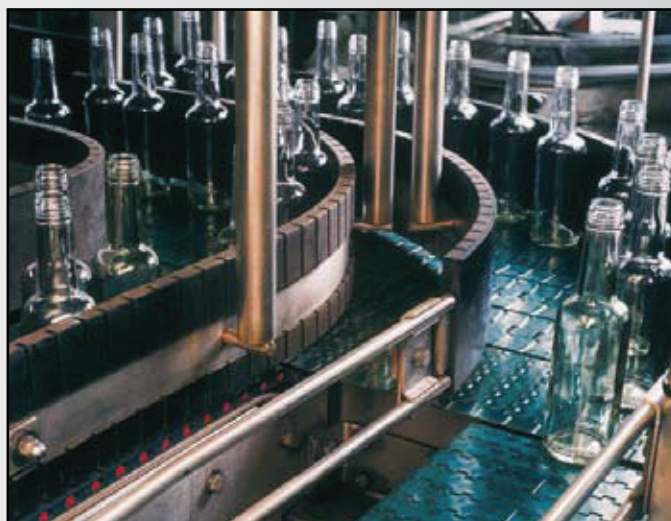
GLASS BOTTLE MANUFACTURING ON 1005 FLAT TOP BELT
