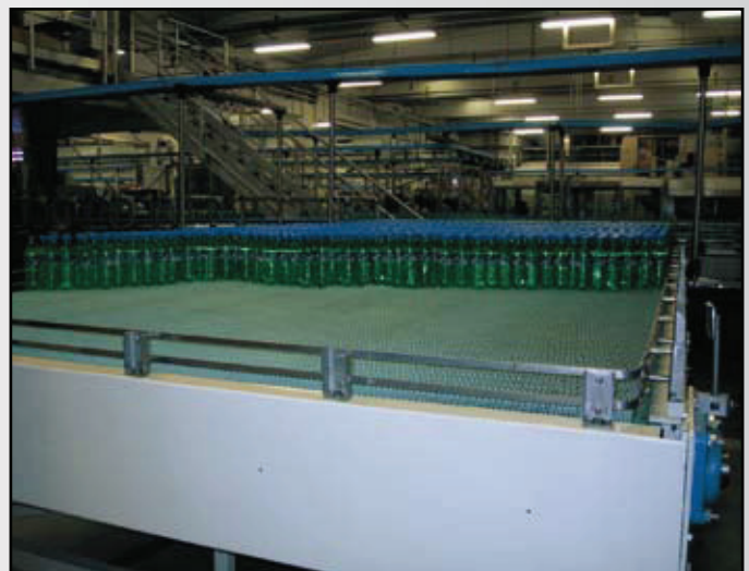
BOTTLE ACCUMULATING ON 2000 BELT
