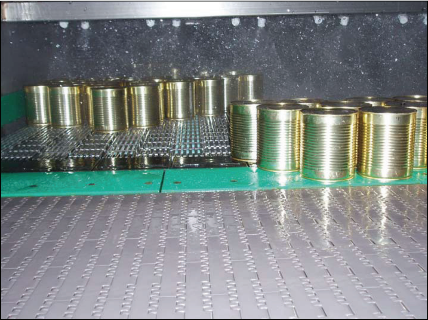
FORTREX 9227 BELT IN A FOOD TUNNEL PASTEURIZER
