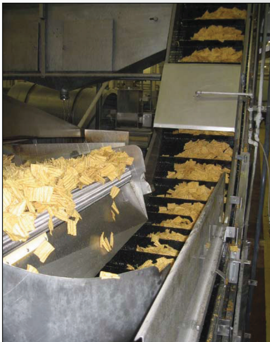
INCLINED CONVEYOR FOR CHIPS FTR2015 BELT
