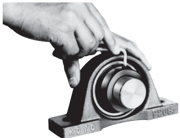
Fig. 14.10 Installing eccentric locking collar
